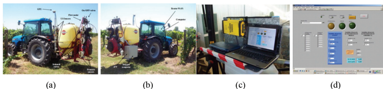
Figure 5. (a) and (b) Placement of components on the sprayer, (c) laptop for wireless control of the prototype from the tractor cab, (d) interface for input data created using LabVIEW [27].
