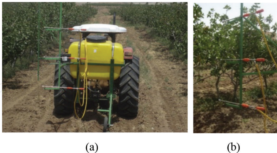
Figure 10. (a) Variable-rate sprayer for fruit tree protection, (b) attached nozzles mounted on the vertical masts for orchard tree spraying [29].
