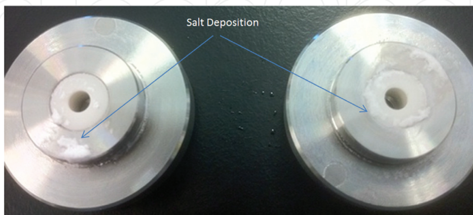
Figure 36. Salt depositions at screws of the column.
