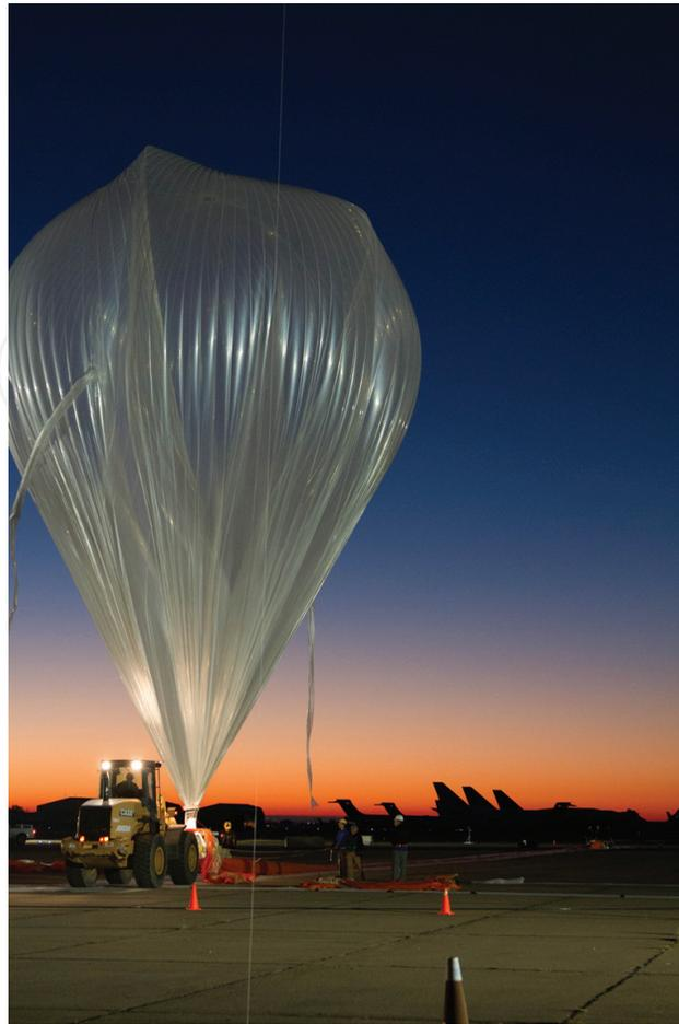
**Figure 5.** The balloon used for the StratEx mission being filled just as dawn breaks. The restraining fabric can be seen tied near the bottom, restricting the fill of the lower part of the balloon.
