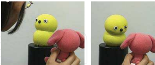
Fig. 7. Keepon engaging in eye-contact (left) and joint attention (right).
