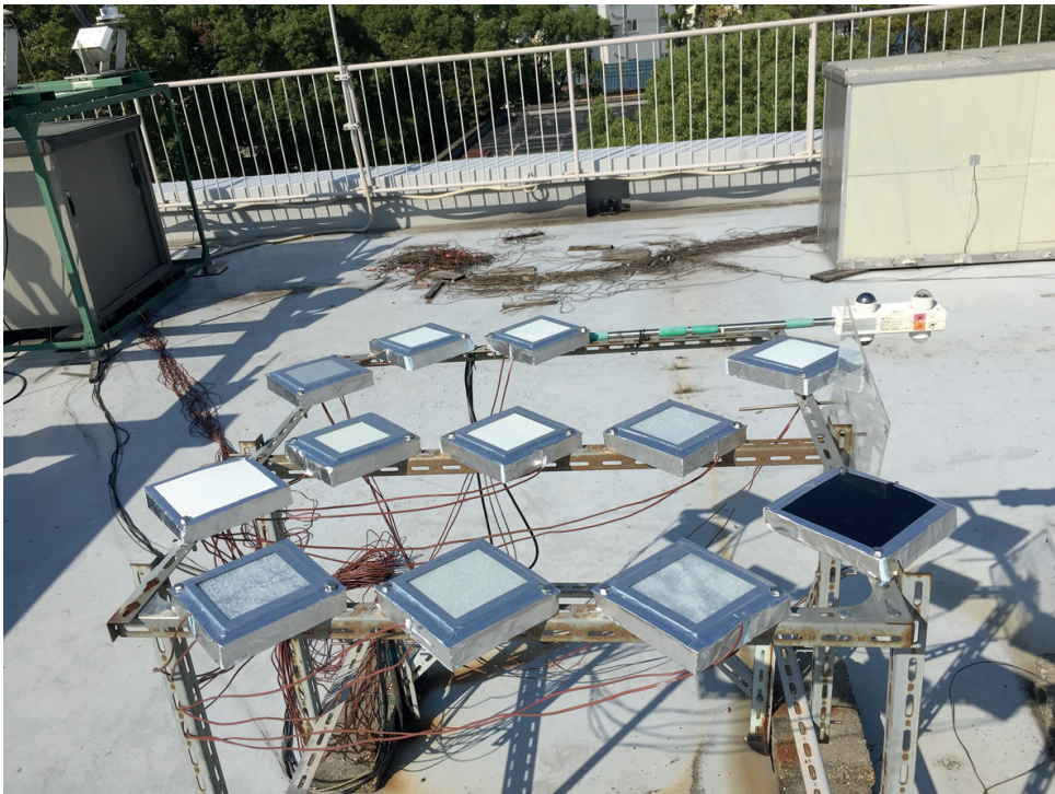
Figure 16. Experimental stand for deriving retroreflectivity of developed glass bead RR samples.
