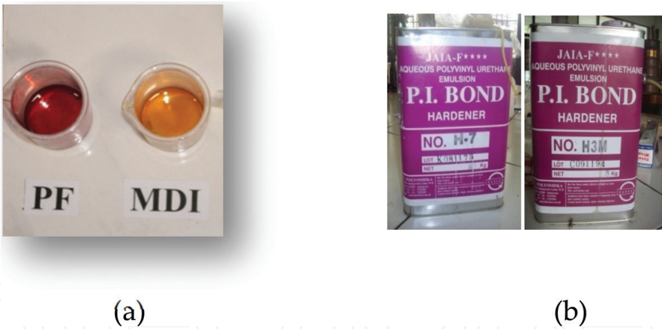
Figure 5. (a) Color comparison between PF resin adhesive and MDI; (b) the isocyanate cross-linker distributed and most used in Indonesia [26, 27].
