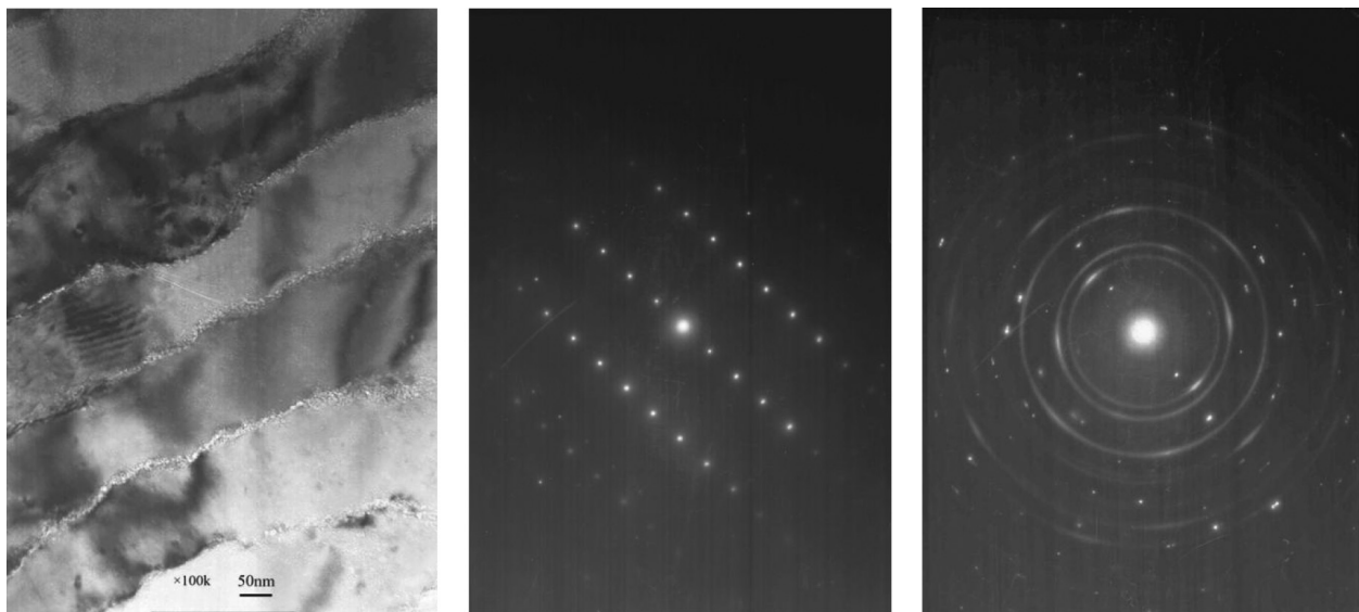
Figure 31. TEM test shows the crystallographic orientations of precious coral sample.
