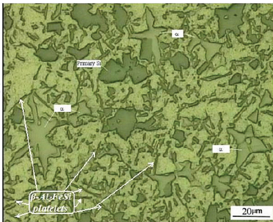
Figure 8. Optical micrograph of al-Si-1.8Fe-0.8Mn microstructure [41].
