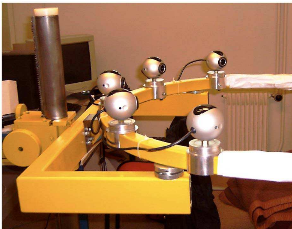
Fig. 1. Acquisition system with the five Logitech cameras fixed on their support
