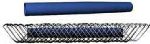
Figure 5. Schematic view of the air muscle
