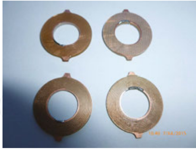
Figure 22. Planar coils corresponding to primary and secondary coils of the microtransformer, INCDIE ICPE-CA concept.
