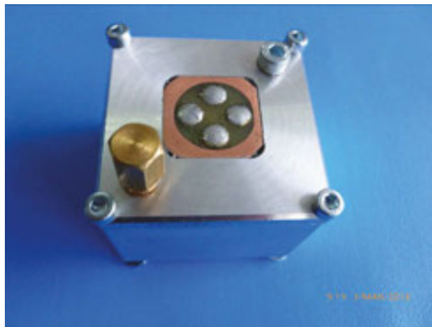
Figure 36. The planar microtransformer with circular spiral windings with hybrid core—ferrite and colloidal magnetic nanofluid, practical achievements.
