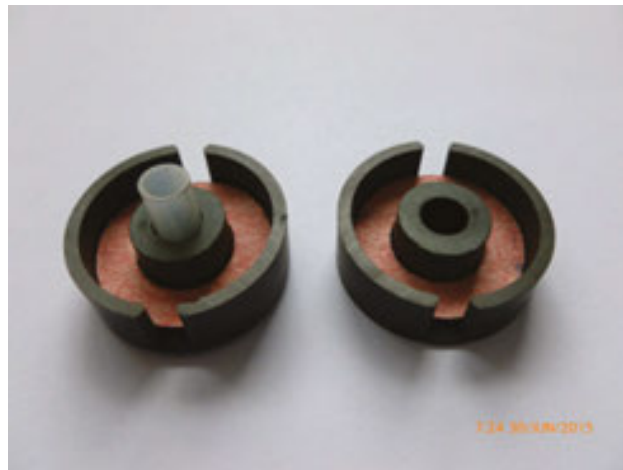
Figure 23. The 3F3 ferrite parts of magnetic circuit.
