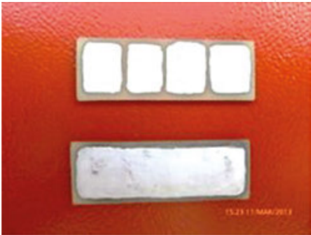
Figure 15. The low energy source built with piezoelectric linear transducers system, INC DIE ICPE-CA concept [26].
