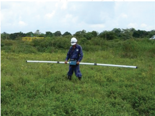
Figure 2. EM31-MK2 ground conductivity meter in field operations [12].
