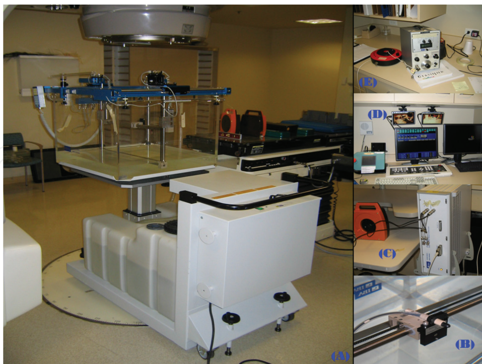
Figure 2. Varian linear accelerator for clinical use, and the basic equipment for radiotherapy calibrations. (A) Computerized water phantom system, (B) PTW ionization chamber N31003 no. 975; (C) Scanditronix Wellhofer; (D) Fixed computer system; and (E) Keithly CNMC electrometer. Courtesy of Dr. Carlos Esquivel, from Cancer Therapy & Research Center, San Antonio, Texas, USA.
