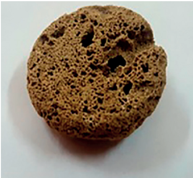
Figure 20. 30% by weight urea-added pellet obtained by microwave irradiation.
