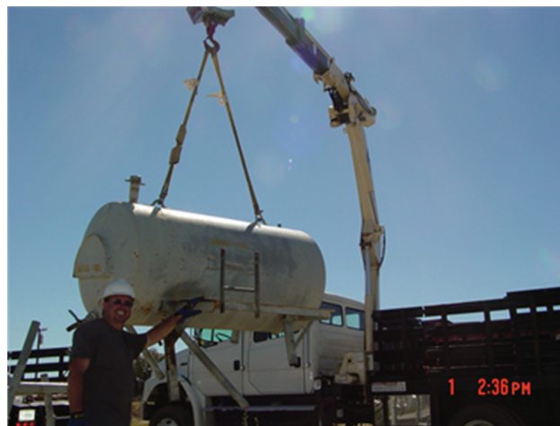
Figure 17. After intervention, truck mounted knuckle boom crane is used in operations where other material handling equipment has not been capable of performing the waste removal.
