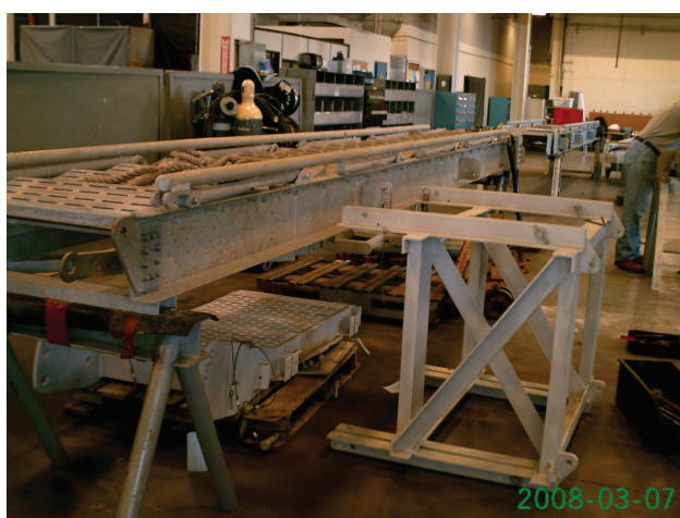
Figure 1. ACCOM ladder on work stands before intervention. The ladders are being disassembled for repair.
