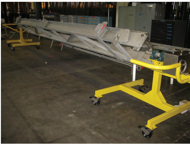
Figure 7. After the intervention, rotating ladder fixture allows one worker to safely turn the ladder and locks into place. The ladder system saves time and effort and reduces the risk of injury and equipment damage.
