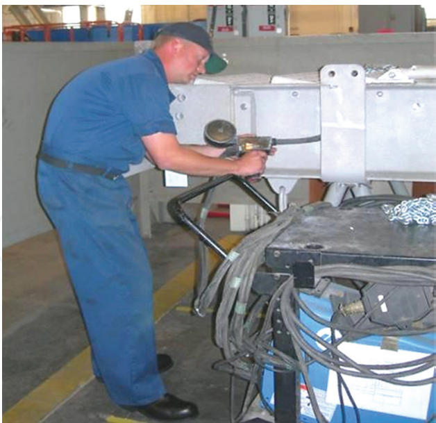
Figure 6. Welder demonstrates awkward postures which were quite common during welding tasks on the ACCOM ladder.
