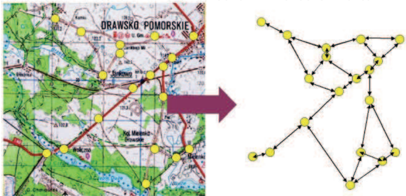
Fig.5. Road-railroad network (left-hand side) and its graph model G_2 (right-hand side)
