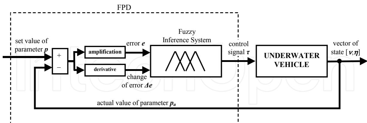
Fig. 4. Block diagram of fuzzy proportional-derivative controller FPD
