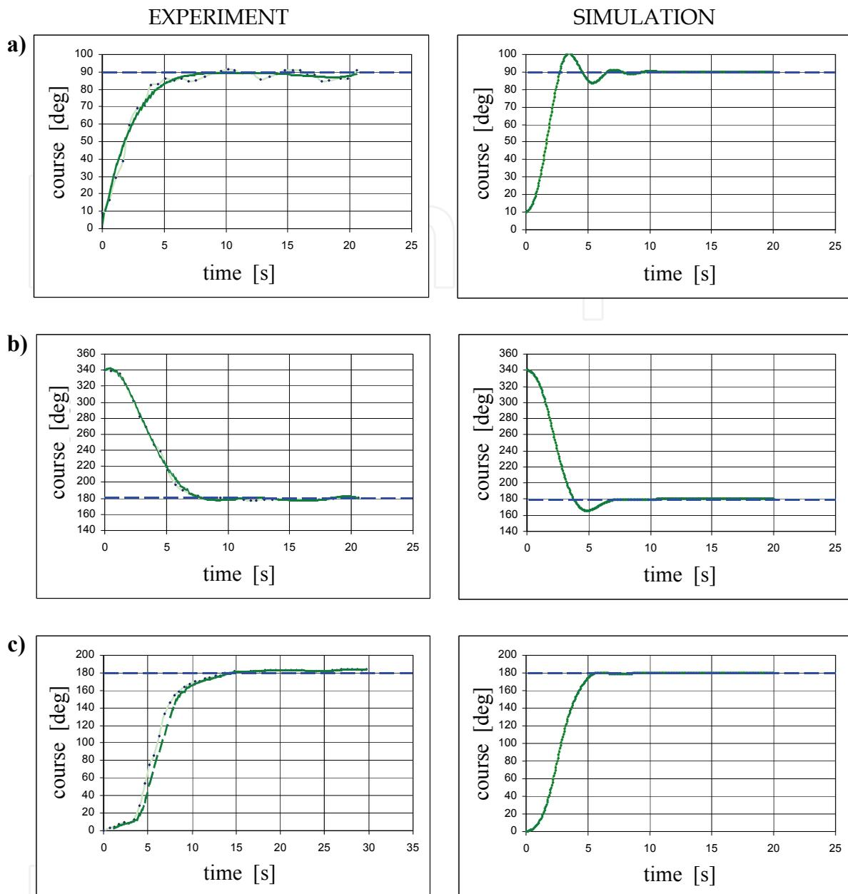
Fig. 11. Control of underwater vehicle's course: a) from initial value  $10^\circ$  to set value  $90^\circ$ , b) from initial value  $340^\circ$  to set value  $180^\circ$ , c) from initial value  $0^\circ$  to set value  $180^\circ$  with additional manoeuvre in X axis
