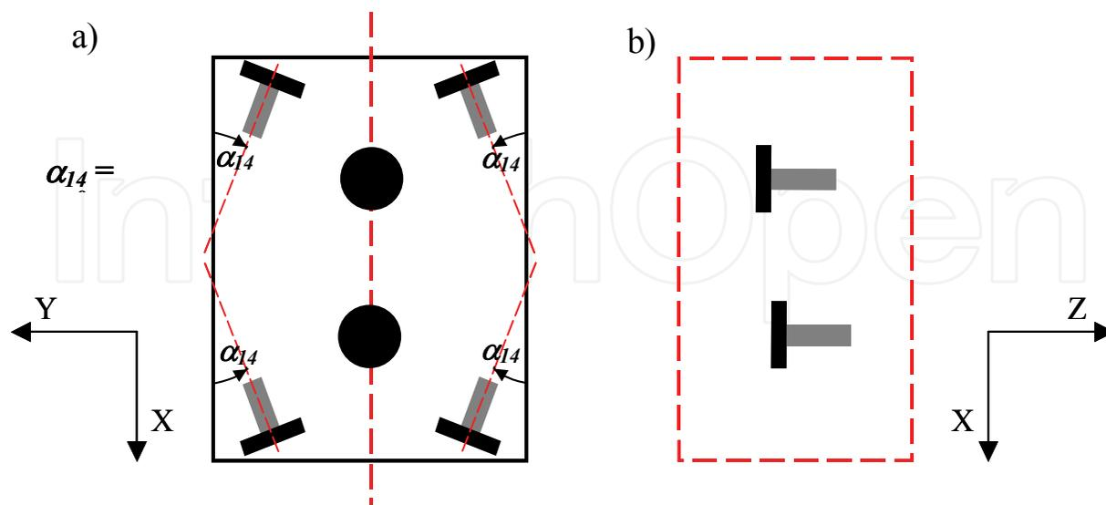
Fig. 2. Location of particular Ukwial's propellers in: a) horizontal and b) vertical plane
