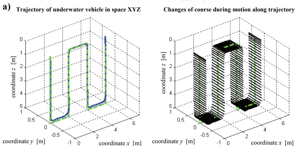
b) Trajectory of underwater vehicle in space XYZ
