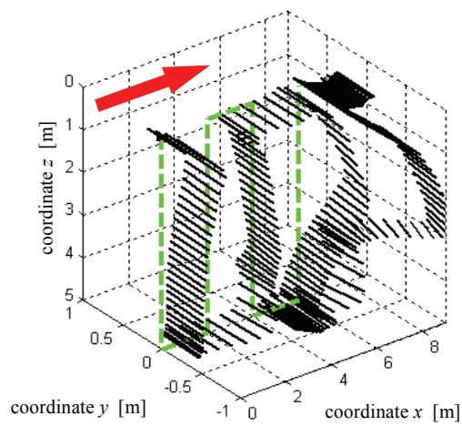
d) Trajectory of underwater vehicle in space XYZ
