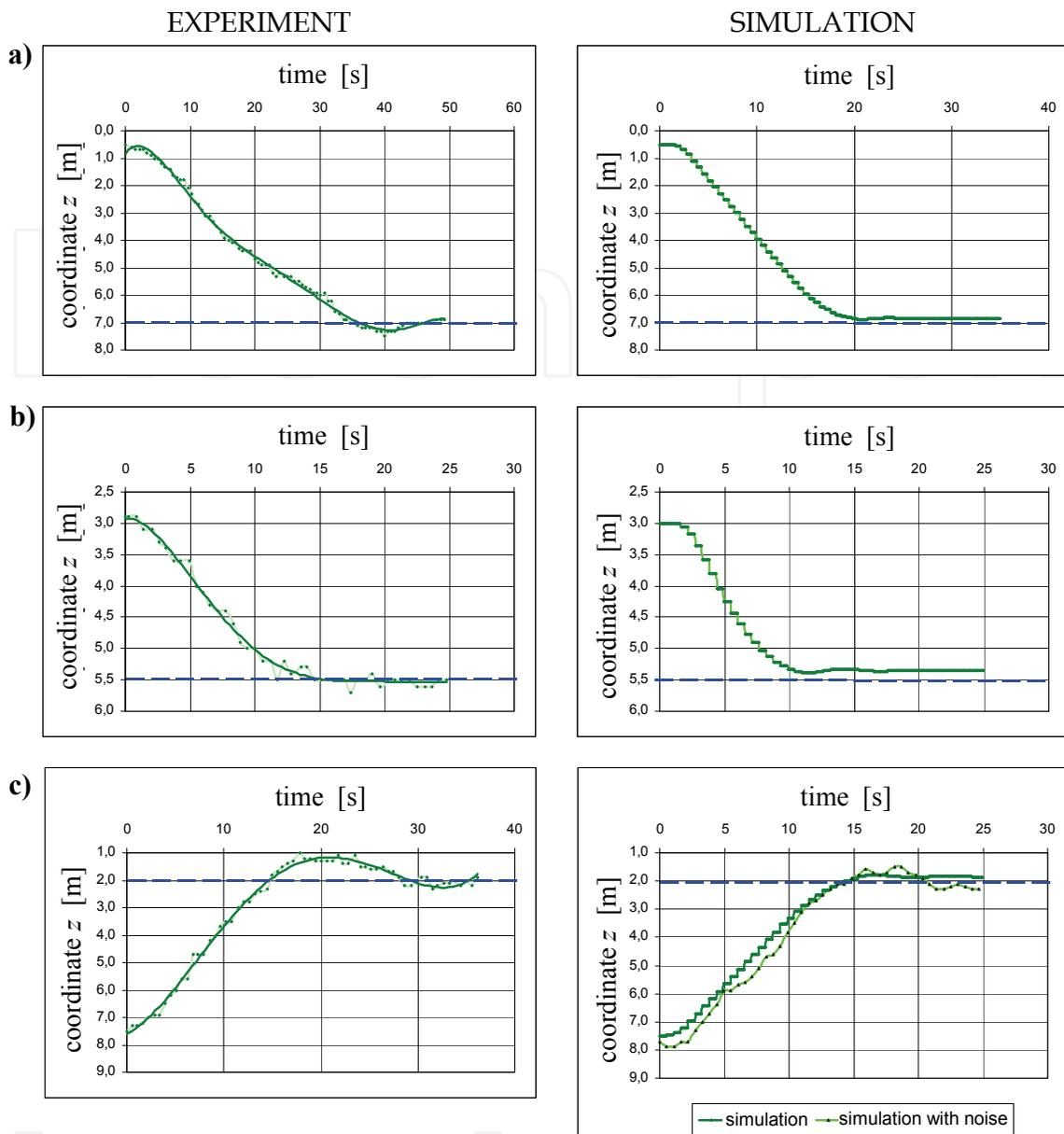
Fig. 12. Control of underwater vehicle's draught: a) from initial value 0,5m to set value 7m, b) from initial value 3m to set value 5,5m, c) from initial value 7,5m to set value 2m (additional simulation with noise)
