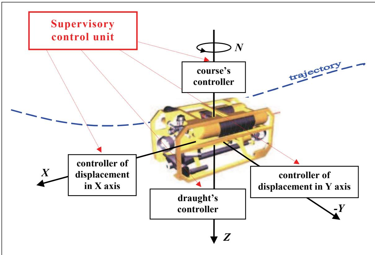
Fig. 3. Automatic control system of underwater vehicle called Ukwiak
