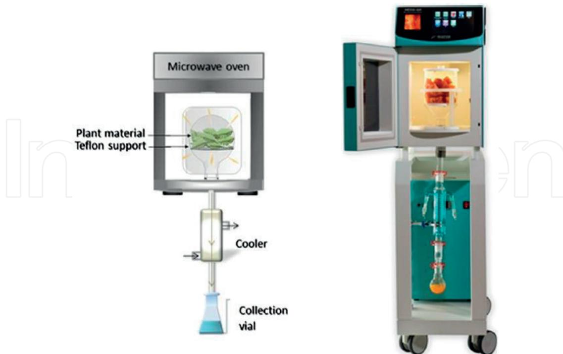
Figure 2. Microwave hydro-diffusion and gravity (MHG) [30].
