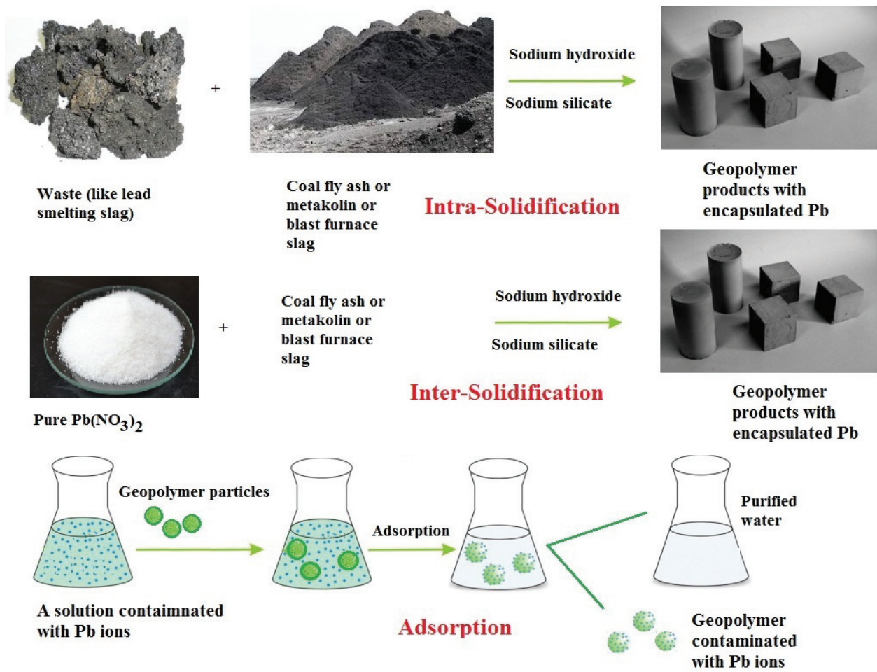
Figure 1. Intra-solidification, inter-solidification and adsorption processes for immobilization of heavy metals.
