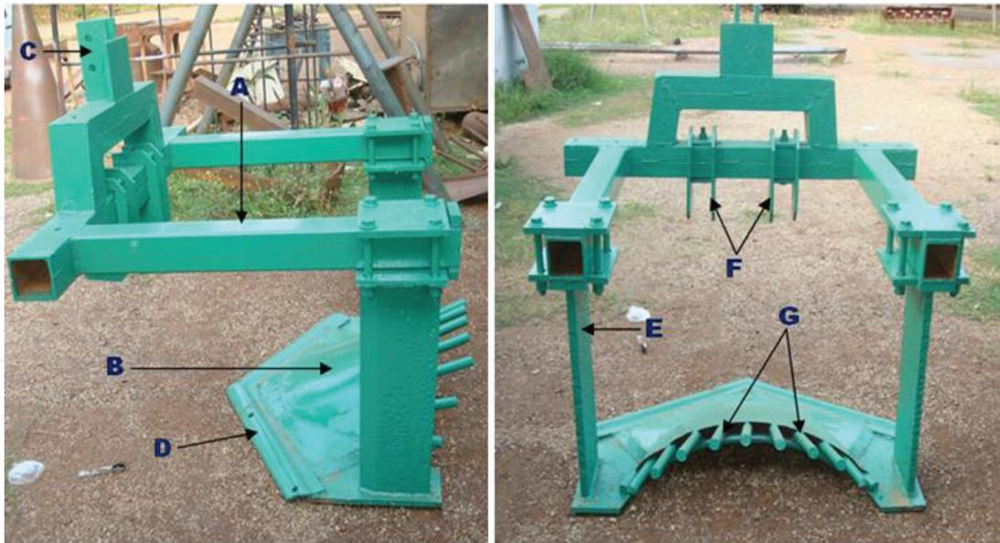
*A – Beam to which digging unit is attached
