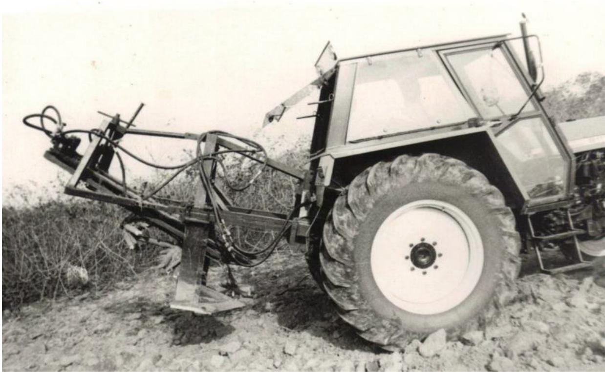
**Figure 5.** The Leipzig mechanical cassava harvester.
