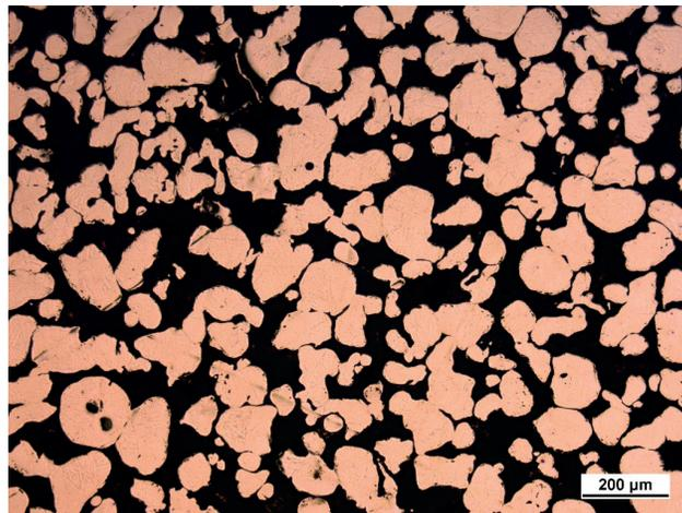
**Figure 7.** Grain size 100  $\mu\text{m}$ , sintering temperature 950°C, sintering time 30 min.
