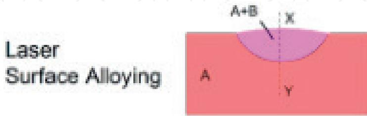
Figure 3. Schematic diagram displaying laser surface alloying [15].
