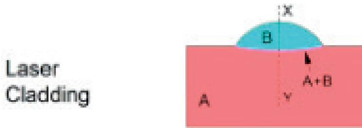
Figure 4. Schematic diagram of laser cladding [15].
