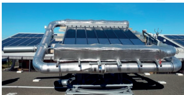
Figure 4. Illustration of the laboratory-scale PVT test rig.
