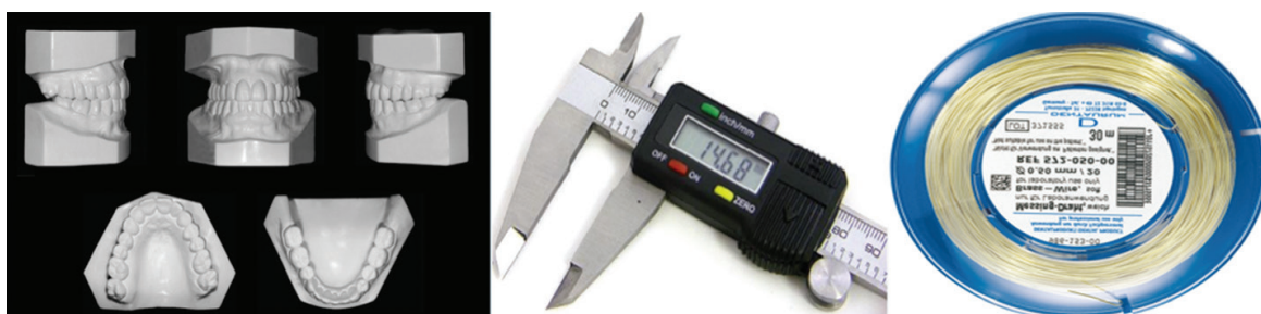
Figure 1. Plaster casts, digital Vernier caliper to performed all measurements and brass wire to measure arch length.
