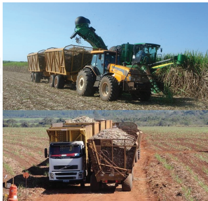
Figure 5. Transshipment to aid the transport of sugarcane from the plot to the truck or train. Credit: Luiz Carlos Dalben.
