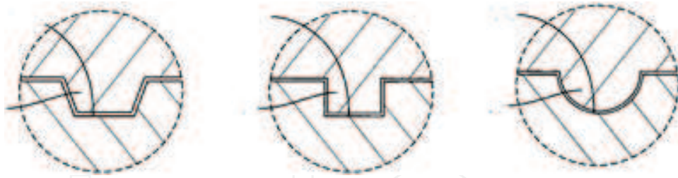
Figure 3. Design features used for self-aligning bipolar plates [17]. Source: United States Patent and Trademark Office, www.uspto.gov .
