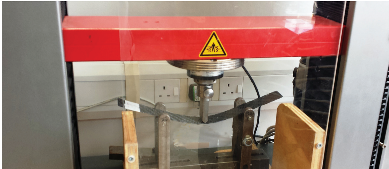
Figure 1. Flexural test equipment: universal testing machine.
