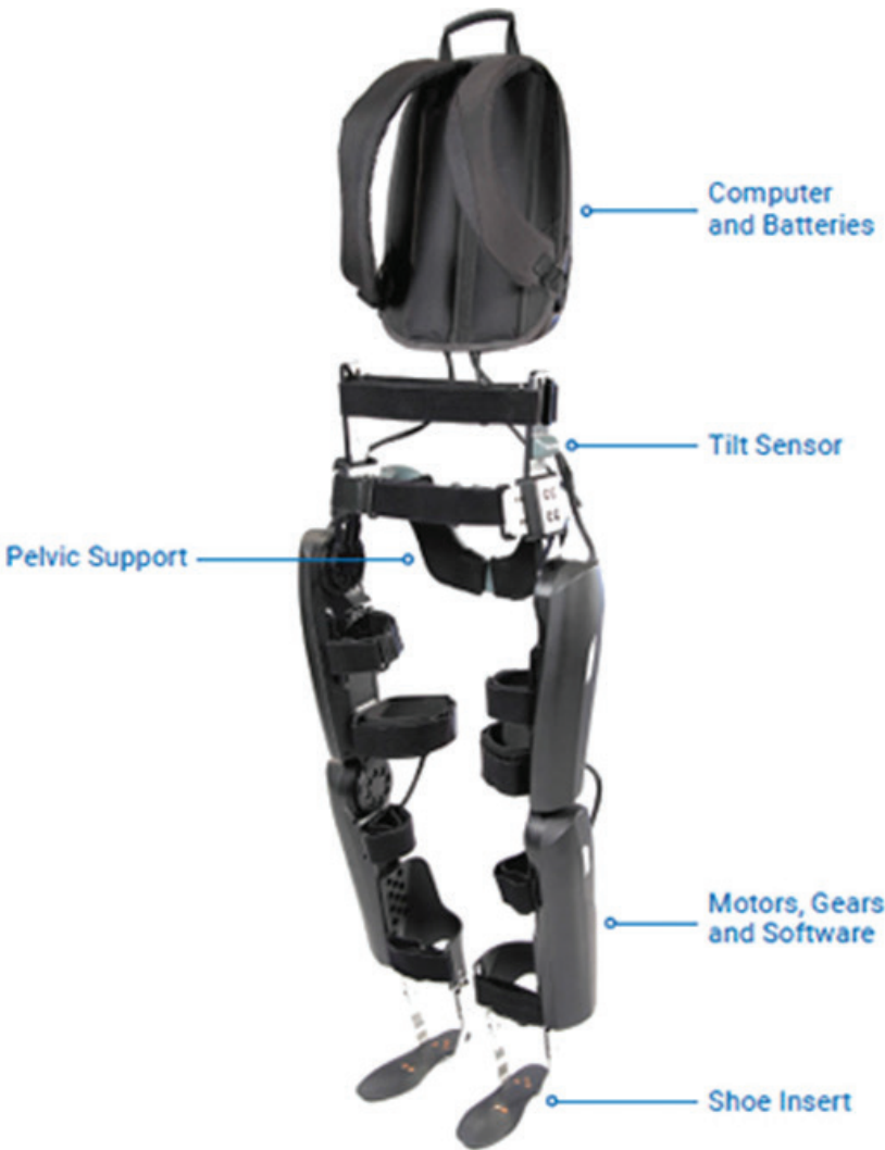
Figure 9. The ReWalk powered orthosis (Argo Medical Technologies).
