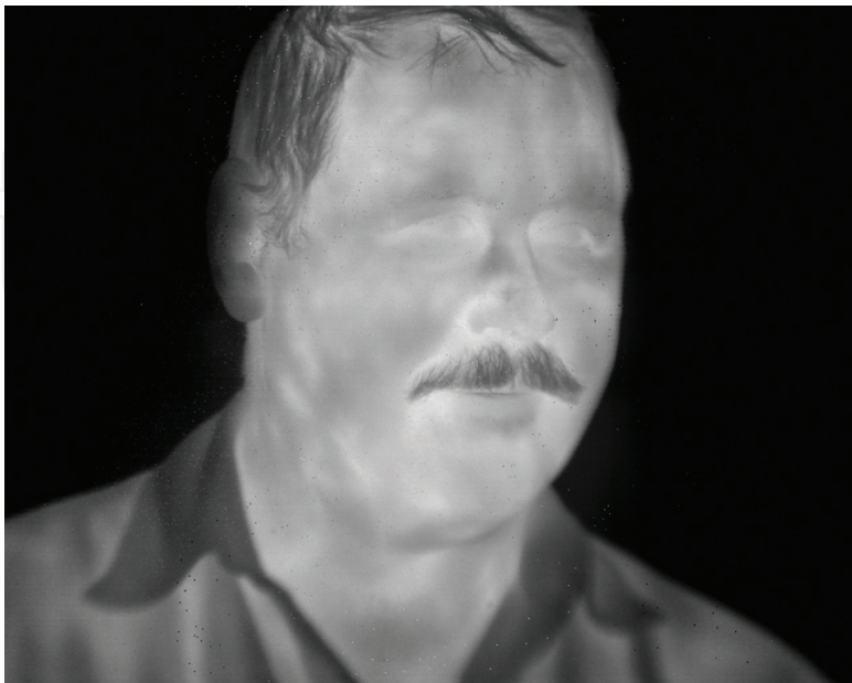
Figure 19. The example of an IR image. The temperature is 65 K. The integration time is 6 ms. The working elements are 99.6%.
