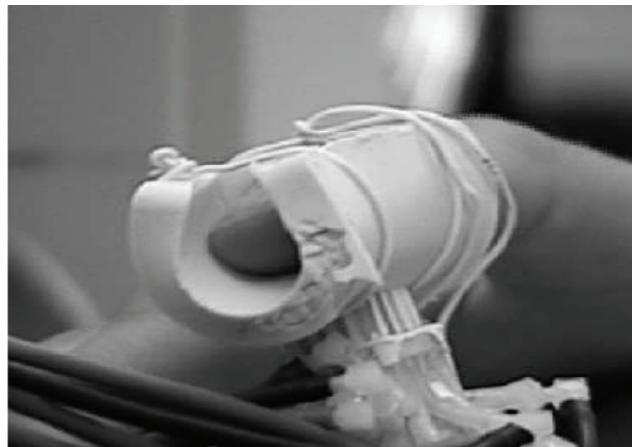
Fig. 7. The softness haptic display attached to the finger
