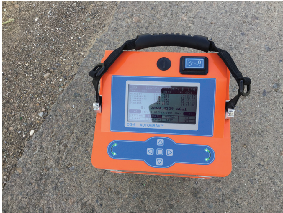
Figure 11. Top view of CG-6 gravimeter during field measurement in Alain city, United Arab Emirates (June 2017) [7].
