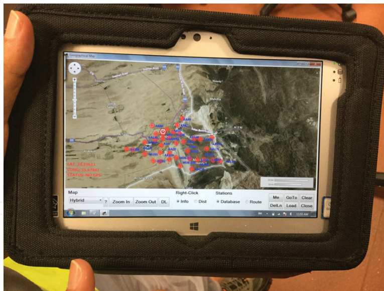
Figure 12. View of lynx LG software (Scintrex, 2017) showing the gravity stations in Alain city, United Arab Emirates, during field survey in Al-Ain city in June 2017. Lynx LG software includes data pre- and postprocessing that helps users to get a simple Bouguer gravity map of the study area just after finishing the measurements [7].
