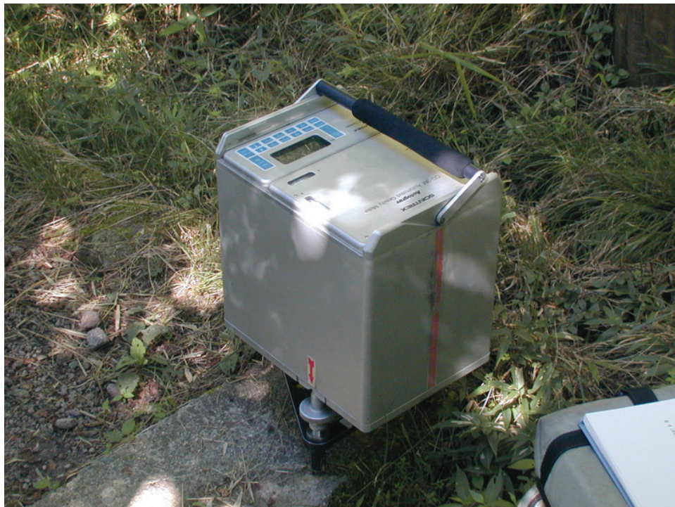
Figure 10. Photograph of CG-3M Autograv automated gravity meter. The features of this gravimeter are: resolution \text{mGal} = 0.001 ( \approx 1 \mu\text{Gal} ), standard deviation: < 5 \mu\text{Gal} , automated corrections: tide, instrument tilt, temperature, and rejection [7].
