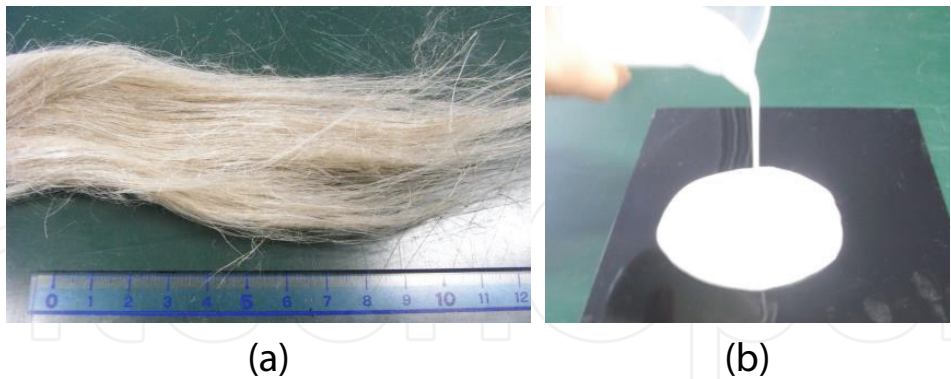
Figure 1. Materials used in this study: (a) as-supplied flax sliver and (b) biodegradable resin.
