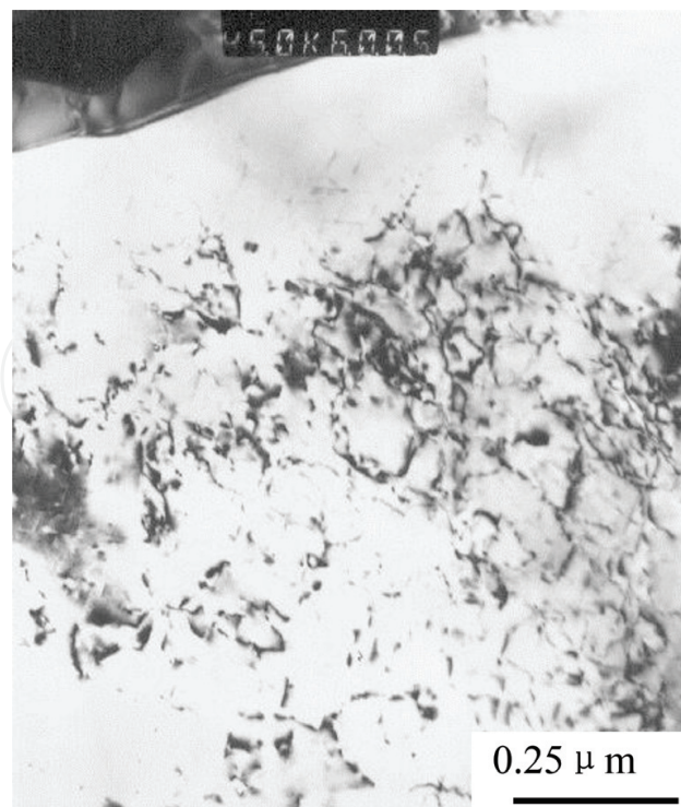
Figure 11. Distribution of dislocations at the interface.
