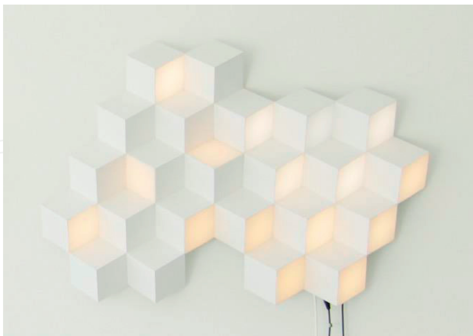
Figure 8. Integrated daylighting and artificial lighting. A close look at a section of the instrument where some surfaces are lit by daylight and some by the embedded LED. The surfaces appear in a range of lit, reflected, and shadowed showing the range of local light variations. Figure 9 shows the same section with the curtains drawn for the window, excluding the daylight.
