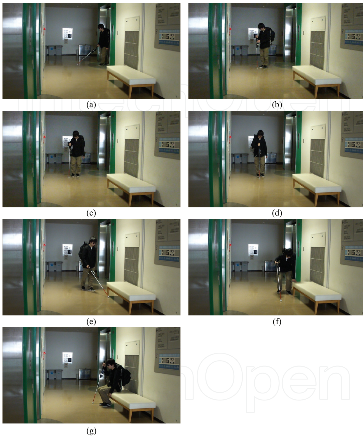
Figure 13. A visually impaired user wants to sit on a bench to take a rest in an elevator hall. (a) A visually impaired user comes out of an elevator. (b) The user instructs the system to find a bench. (c) The user pans the Kinect sensor. (d) The system finds the bench. (e) The user walks toward the bench. (f) The user confirms the bench. (g) The user can sit on the bench.
