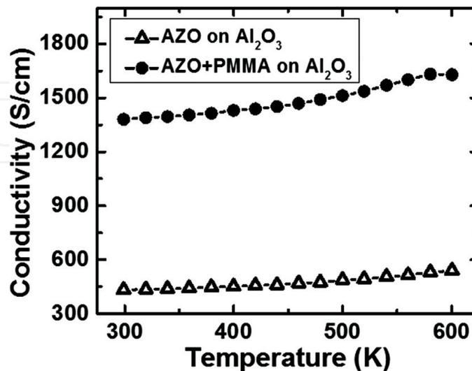
**Figure 6.** Temperature dependence of the electrical conductivity of AZO and AZO + PMMA films deposited on Al<sub>2</sub>O<sub>3</sub> substrates.
