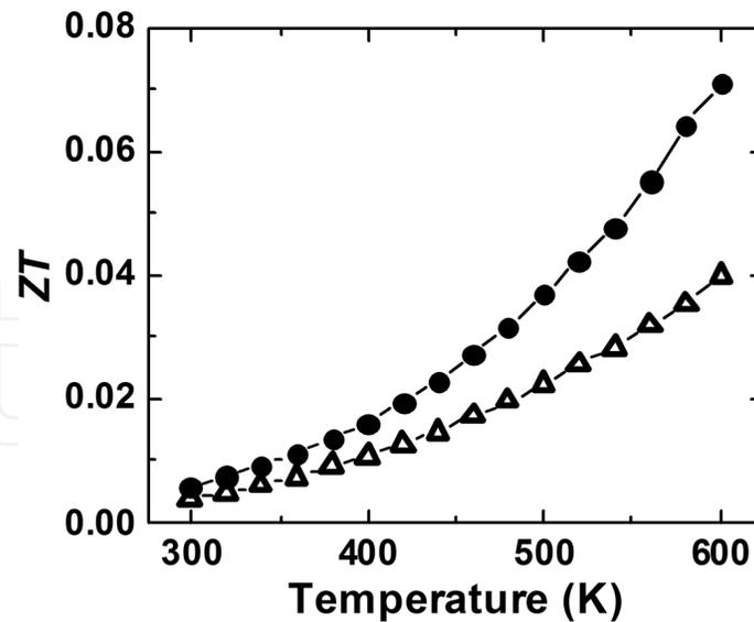
**Figure 11.** Temperature dependence of the thermoelectric figure of merit  $ZT$  of AZO and AZO + PMMA thin films on  $\text{Al}_2\text{O}_3$  substrates. Symbols used to represent data points are the same as in **Figure 6**.  $ZT$  was calculated using the thermal conductivities of AZO and AZO + PMMA films on  $\text{Al}_2\text{O}_3$  substrates measured at 300 K (see **Table 1**).
