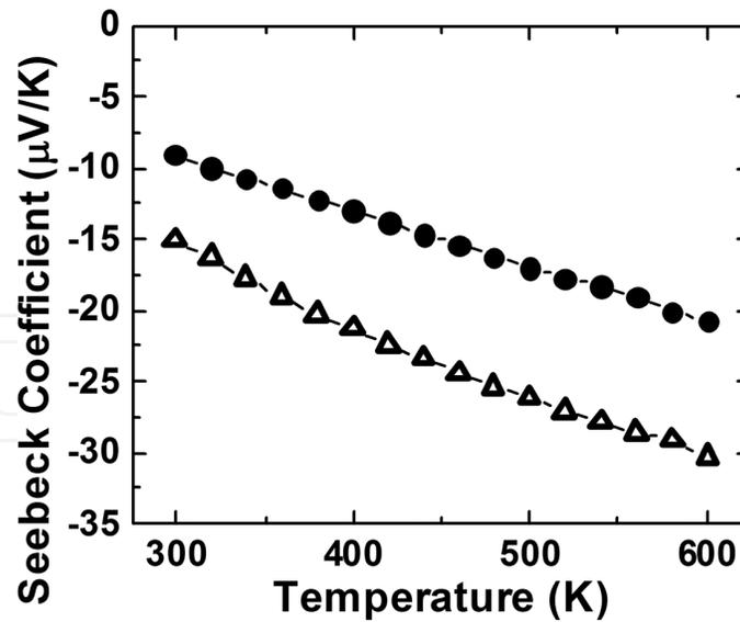
**Figure 7.** Temperature dependence of Seebeck coefficient of AZO and AZO + PMMA thin films on Al<sub>2</sub>O<sub>3</sub> substrates. Symbols used to represent data points are the same as in Figure 6.
