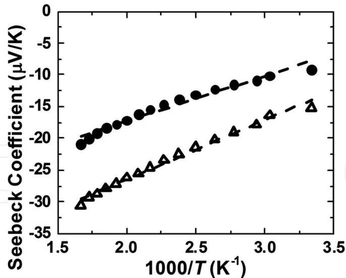
**Figure 10.** Inverse temperature dependence of Seebeck coefficient of AZO and AZO + PMMA films on Al<sub>2</sub>O<sub>3</sub> substrates. Dashed lines are the linear fit of the corresponding plots. Symbols used to represent data points for different samples are the same as in **Figure 6**.
