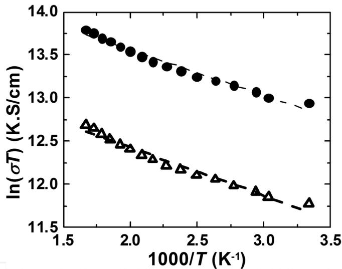
**Figure 9.** Inverse temperature dependence of  $\ln(\sigma T)$  of AZO and AZO + PMMA thin films on  $\text{Al}_2\text{O}_3$  substrate. Dashed lines are the linear fit of the corresponding plots. Symbols used to represent data points for different samples as in Figure 6.
