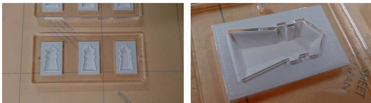
Figure 13. 3D printing mold of 3D Tateyama apple RAKUGAN.
