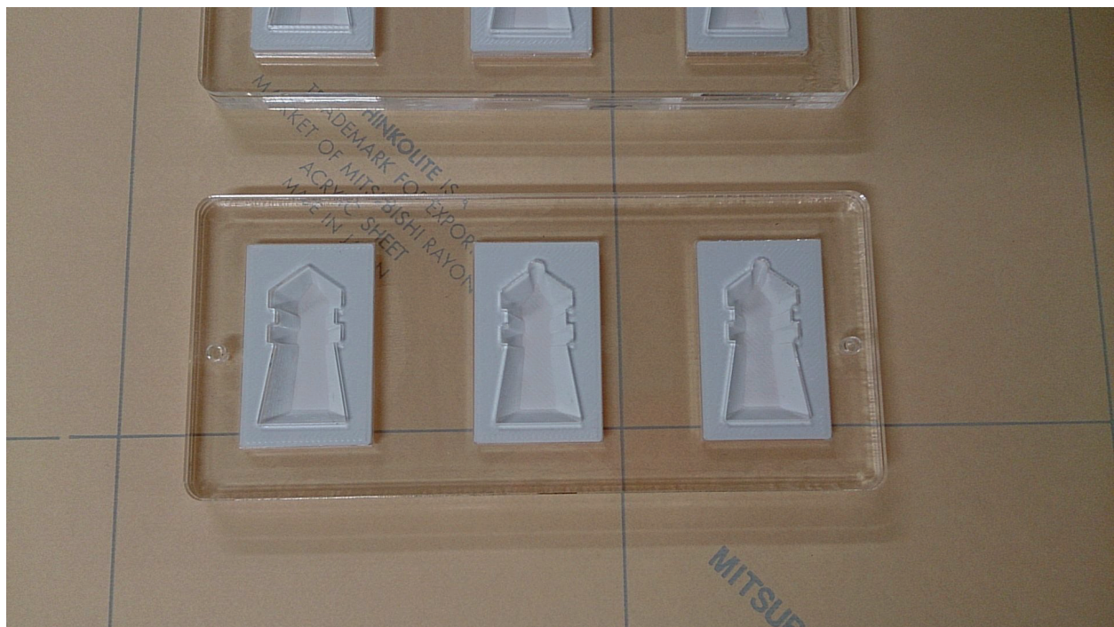
Figure 4. 3D printing mold of “3D Tateyama apple RAKUGAN”.
