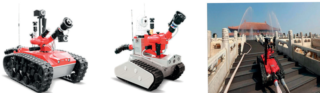
Figure 14. The fire-fighting robot and tests.
