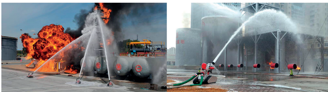
Figure 15. The high temperature protection tests of the fire-fighting robot.
