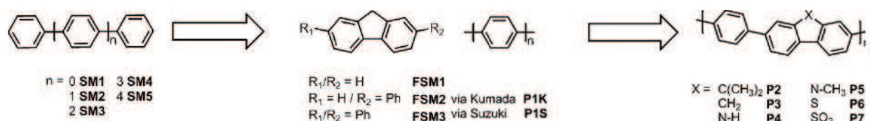
Figure 11. Schematic representation of reactions for the synthesis of planarized conjugated polymers. Reproduced with permission from Wiley-VCH; see Ref. [46].
