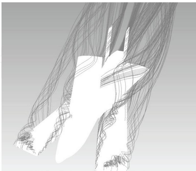
Figure 13. Vortices from rear wings go on forward wings (rotation angle 15^\circ , angle of attack 24^\circ ).
