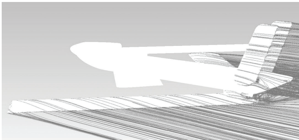
Figure 15. Flow separation after fin (rotation angle 30^\circ , angle of attack 0^\circ ).
