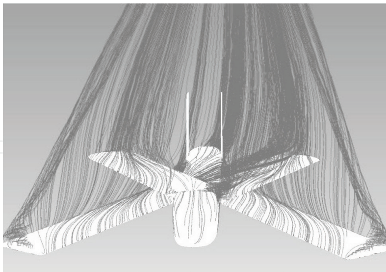
Figure 12. Vortex over forward left wing (rotation angle 15^\circ , angle of attack 24^\circ ).
