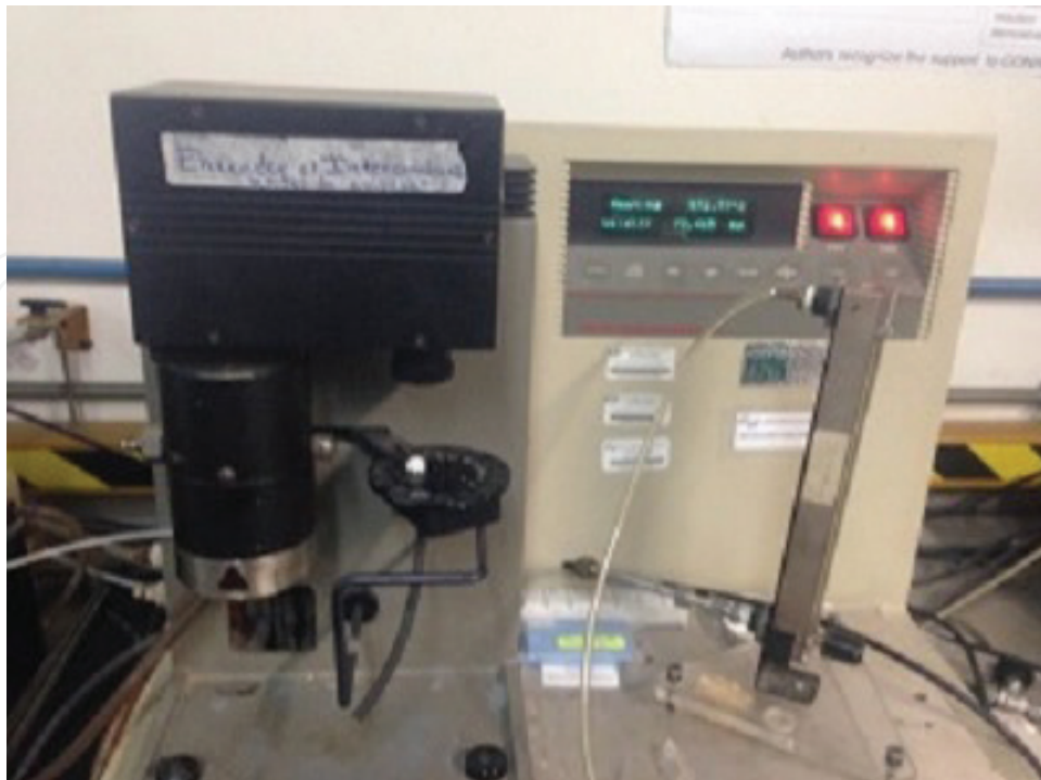
Figure 2. Thermogravimetric analyzer TA Instruments.
