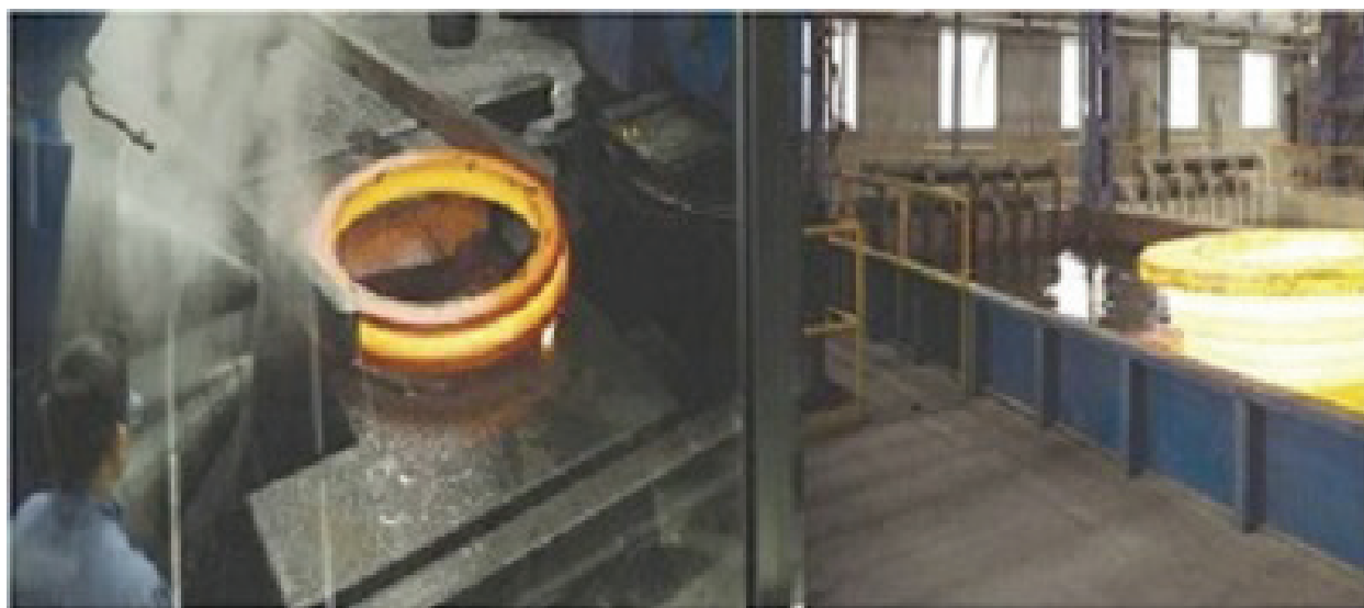
Figure 1. Seamless rolled rings for aircraft engines [6].
