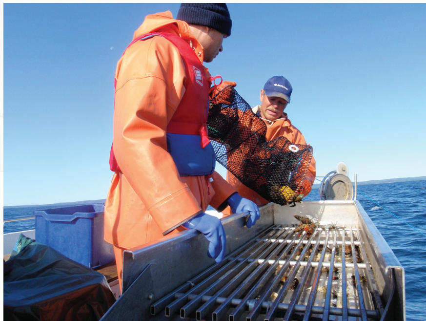
Figure 2. Sorting of crayfish catch on board by size. A system of a grid with expanding distances of metal bars allows crayfish to be sorted by size as they slide on the grids. Photo by MSc Fredrik Engdahl (SLU Aqua, Sweden).
