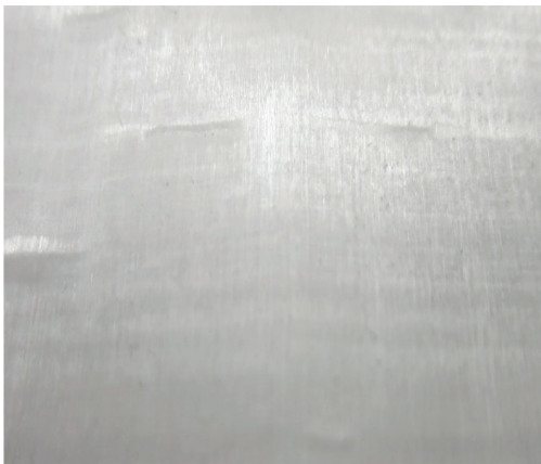
Figure 11. Ballistic panel Spectra Shield® SR-1226 by Honeywell; source: author’s own photo archives. Note: Sample is composed of two panels and each of the panels consists of two layers. The first layer consists of sets of the parallel yarns positioned vertically (V) and the second layer contains the parallel yarns positioned horizontally (H). Thus, the scheme of the sample construction is: (V + H) + (V + H). Total area density: 253 g/m 2 . Thickness: 0.7 mm.
