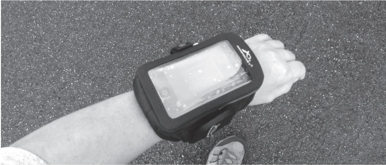
**Figure 4.** Mounting of the smartphone as a wireless gyroscope platform for quantifying reduced arm swing [49].
