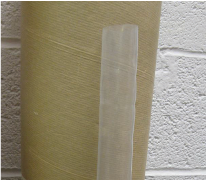
Figure 4. Flexible transparent plastic tubing used to cast glass beads.
