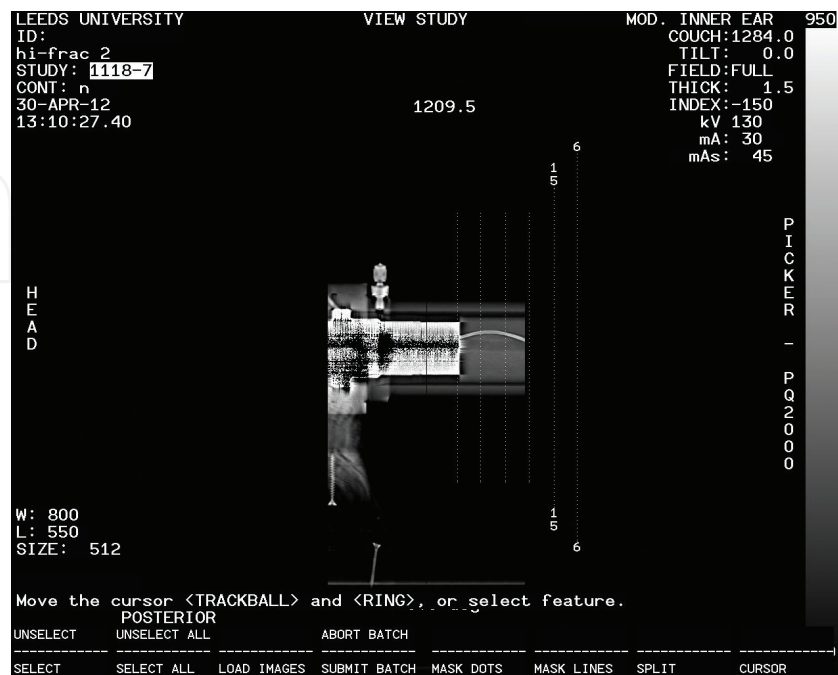
Figure 21. Longitudinal layout of the core holder containing the limestone specimen.
