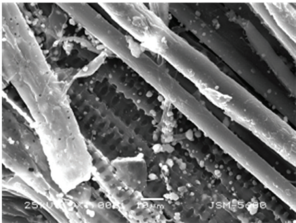
Figure 9. Morphologies of tensile fracture of (a) the bamboo fiber treated with alkaline solution; and (b) the untreated bamboo fiber.
