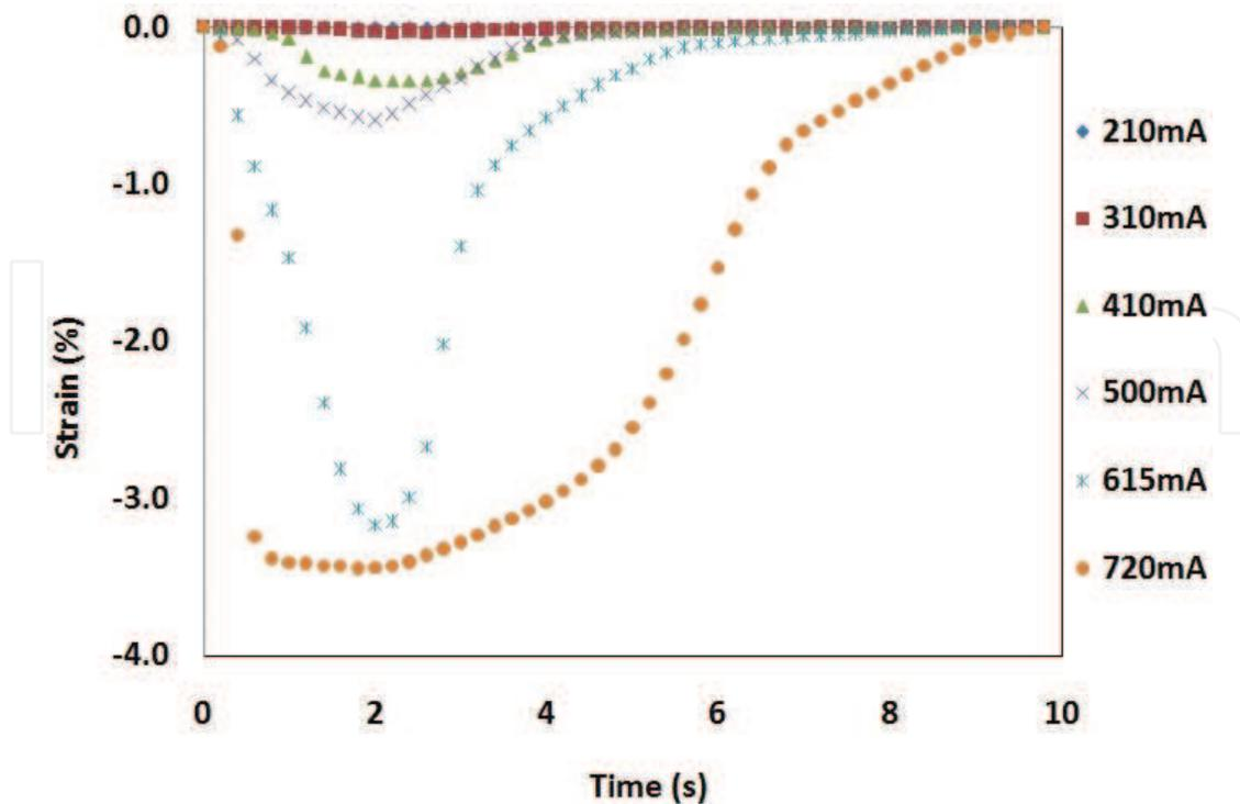
Figure 8. SMA actuator response against 2 seconds actuation in grease.
