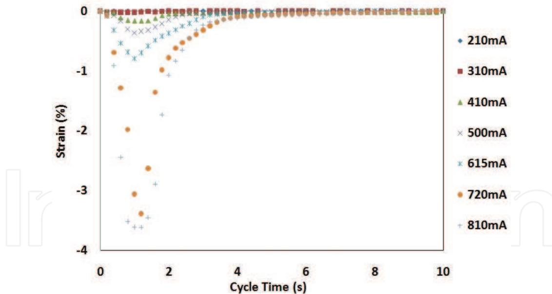
**Figure 7.** SMA actuator response against 1 second actuation in grease.
