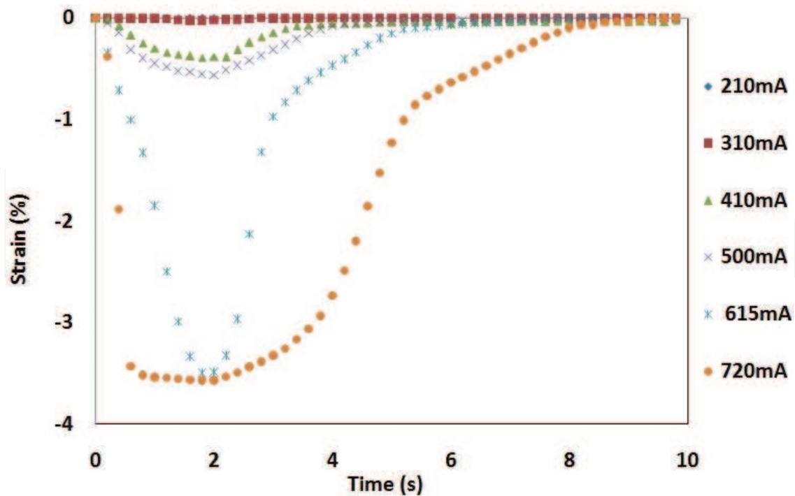
Figure 10. SMA actuator response against 2 seconds actuation in oil.
