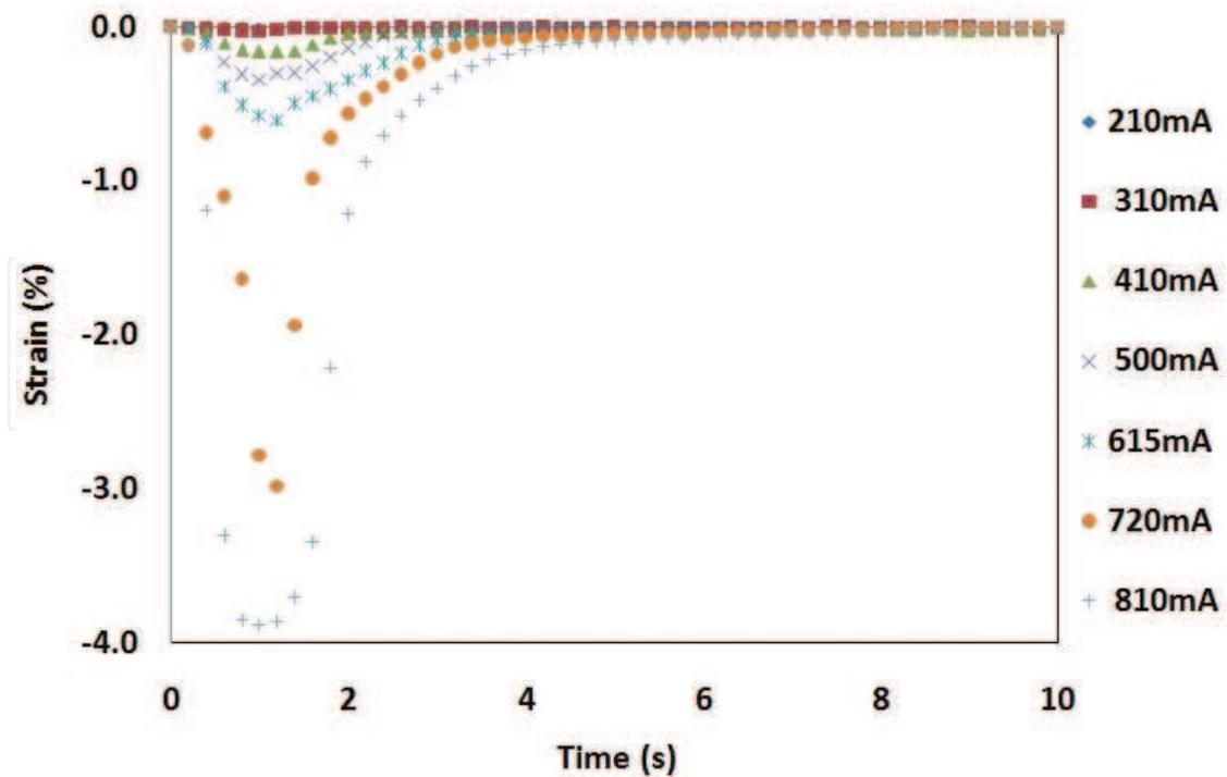
Figure 9. SMA actuator response against 1 second actuation in oil.
