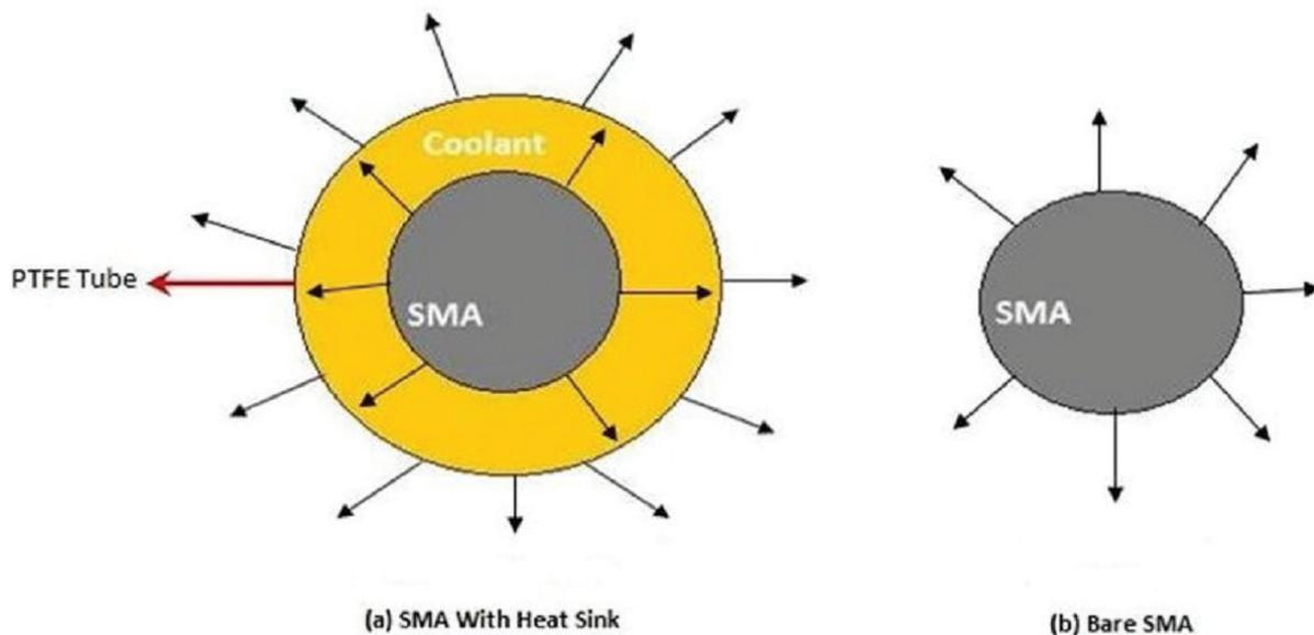
**Figure 5.** Area and heat dissipation model of (a) SMA with sink and (b) bare SMA.
