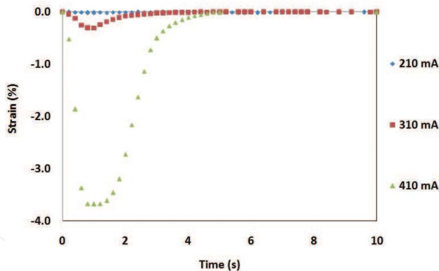
**Figure 6.** SMA actuator response in ambient air.
