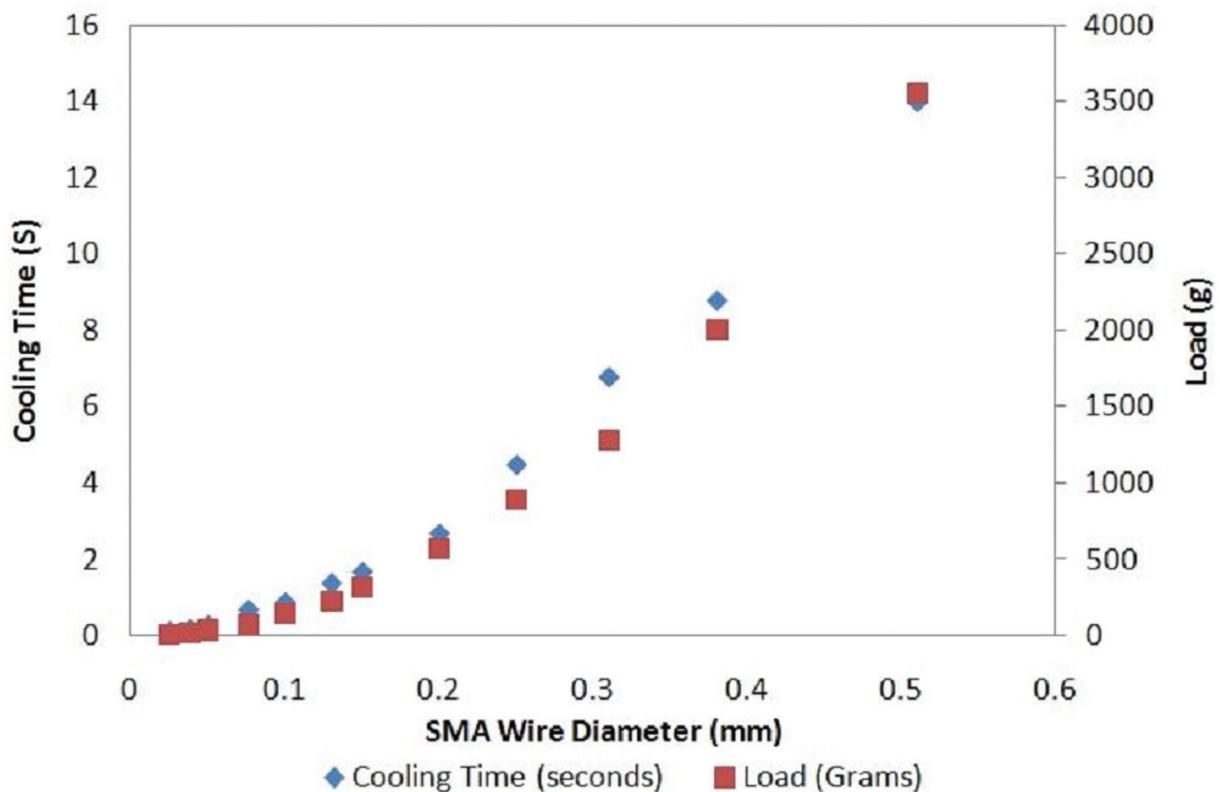
**Figure 2.** Relationship between wire diameter, cooling time and safe load for SMA wire actuators.
