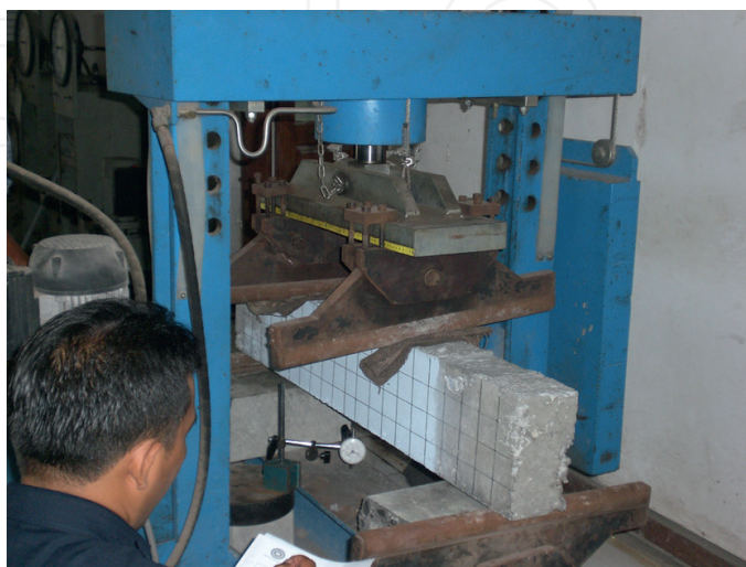
Figure 4. The loading test of concrete beam which 120 mm \times 250 mm with the reinforcement area were 400 and 1200 mm 2 [22].
