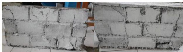
Figure 6. Collapse of concrete block wall sample after being tested [3].
