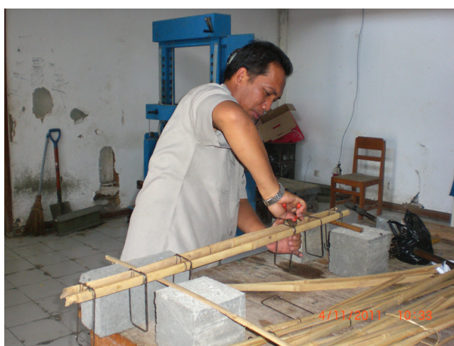
Figure 3. The bamboo reinforced concrete beam assembled was 120 mm \times 250 mm. The reinforcement area were 400 and 1200 mm 2 [22].
