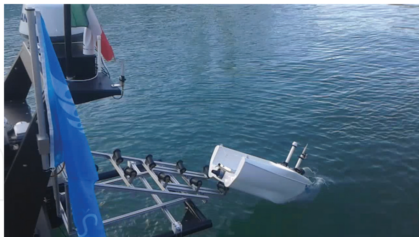
Figure 14. UCAP being launched from the U-RANGER (source: ICARUS).
