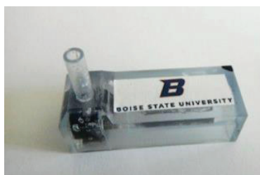
Figure 28. Micro-pump created based on Ni-Mn-Ga alloys [111].
