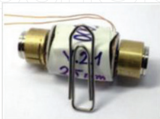
Figure 29. Energy harvester based on MSM alloys developed by Adaptamat [109].
